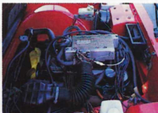
Transmission tunnel dominates; 2.8-litre Cologne V6 gives 160bhp
